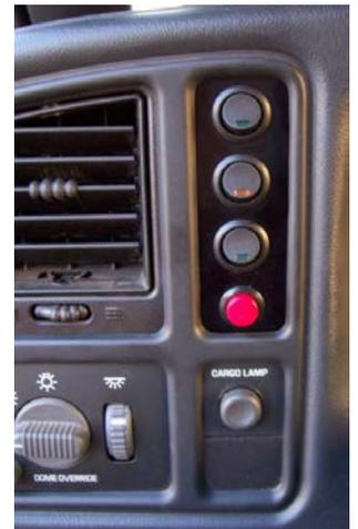
**Step 7:** Test the system and make sure your wiring is correct. With the key in the on position turn on system arm, the solenoids should click. If they don't something is wired wrong. If they do click then turn on the heater and see if it gets warm, then try your purge. Once everything is working correctly move to the next step.
