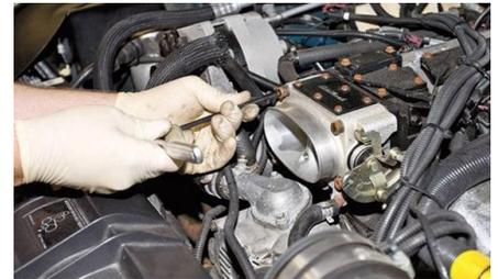
**Step 4:** Remove your stock linkage bracket. Install the 3 extension brackets using the 3 hex head bolts in your kit and hand tighten. Make sure to keep your extension brackets as flat as possible to keep the throttle cable bracket alignment.
