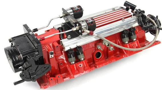
**Step 8** Most late model EFI GM vehicles will have a 4AN schrader valve that you can tap into on the stock fuel rail to feed your fuel solenoid, you will need to remove the valve in the fitting using a schrader valve tool or a small screw driver. If your vehicle does not have a schrader valve or you have aftermarket fuel rails you will need a manifold or fuel rail adapter. It helps to have a rag handy to catch spilled fuel.
