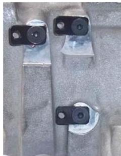
Linkage extension brackets installed. Must be aimed forward and straight. Tighten the counter sunk bolts.
