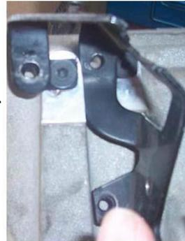
Reinstall stock bracket using stock bolts. You must grind a little material away from the bottom bolt area and just below the 2nd bolt area, so that the bracket can move forward.
