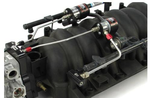
78mm FBody/GTO/Corvette plate fittings face back toward the firewall
