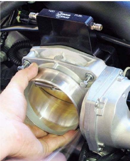
**Step 7** Tighten all (4) bolts on the throttle body.
