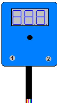
**Switch #1** - toggles through the configuration menu. As you toggle through the configuration menu, the stored value will be displayed. Each time you push Switch #1 it will move the flashing character to the next digit. EXP. Space "B" will be flashing while making changes to this field (using switch 2), push switch 1 when you are ready to move to space "C" Each step is programmed the same way.
