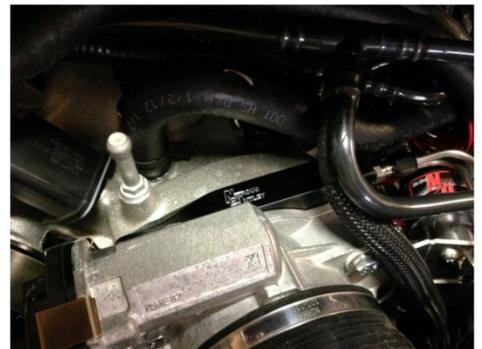
**Step 9** Connect the vacuum hose back to the throttle body. Then plug back in the TPS and IAT sensors. After everything is reconnected attach the cold air tube back to the the throttle body.
