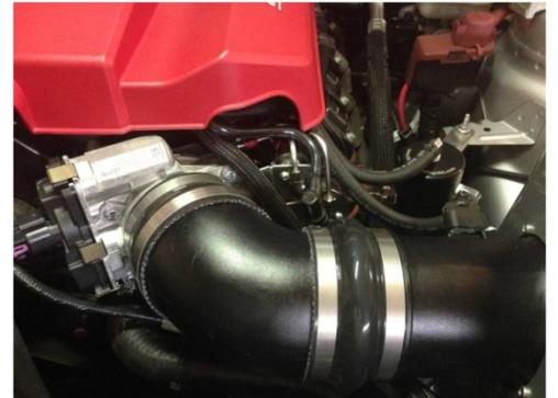
**Step 7** Tighten all (4) bolts on the throttle body.
