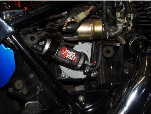
With the "T" fitting installed, use the rubber fuel line and clamps that are included in your system to connect to "T" fitting to the inlet nipple of the enclosed fuel filter, use the rubber hose and clamps to connect the outlet of the fuel filter to the inlet of the fuel pump. Now, use the enclosed rubber hose and clamps to connect the outlet nipple of the fuel pump to the fuel solenoid inlet nipple. Double check all your fuel line connections and clamps.
