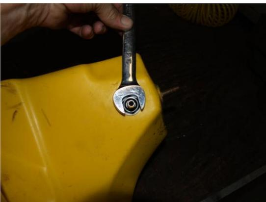
Next, place the enclosed white Teflon washer on the threaded portion of the fitting protruding out of the tank, thread the nut on. Do not over tighten the nut. Install the barbed fitting into the of the outlet assembly using thread sealant on the pipe threads. It might be necessary to hold the fitting on the inside of the tank in order to properly tighten the outlet nipple. Reinstall the stock fuel pump, reinstall the tank on the vehicle, fill with fuel and check for leaks. Use the
