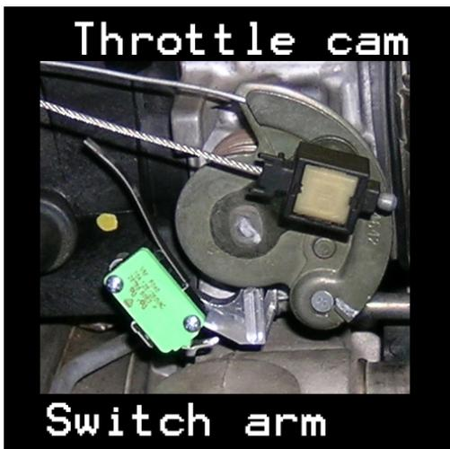
Step 3: Reinstall the bracket and bolt, as shown, making sure the alignment between the throttle cam and the switch arm is straight. Use your 10mm wrench or socket/ratchet to torque to OEM mfg specs.
