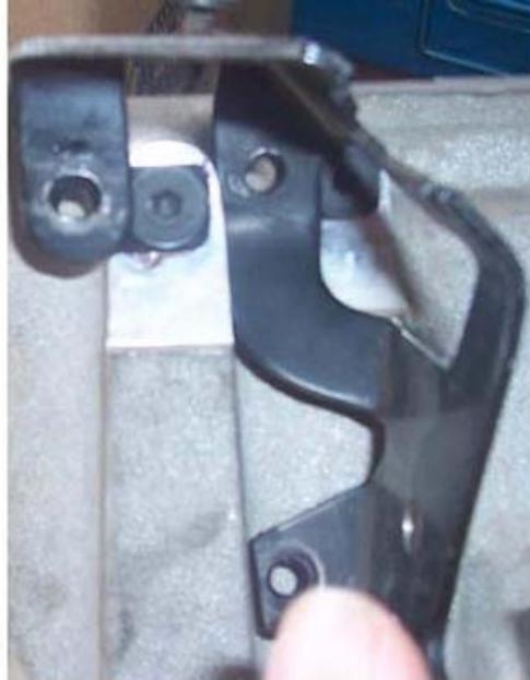
**Reinstall stock bracket using stock bolts. You must grind a little material away from the bottom bolt area and just below the 2nd bolt area.**
