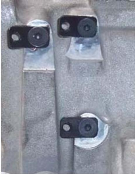
**Linkage extension brackets installed. Must be aimed forward and straight. Tighten the counter sunk bolts tight.**
